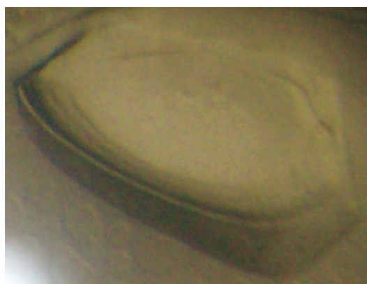
Figure 2 Crystal (dimensions 0.3 × 0.2 × 0.05 mm) of filamin A repeats 14–16 in 1.6 M ammonium sulfate, 2% PEG 1000 and 100 mM HEPES pH 7.5. Although lacking distinct edges, this lens-shaped crystal diffracted to 1.7 Å.
